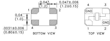
Chamfer on PIN 1 (Default)
